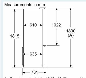
**A:** Front is adjustable 1830–1847 mm, with front levelling feet fully extended
