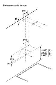
$\ensuremath{\mathbf{B}}\xspace$  : Gas - from upper edge of pan support C: Electric - for Australia and New Zealand
