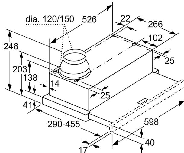
Depth of the filter drawer can be adjusted by up to 29 mm
