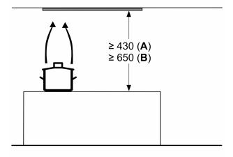
from upper edge of pan support **A:** min. 430 electric **B:** min. 650 gas
