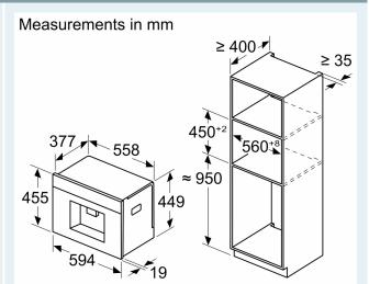
Bean and water containers are removed from the front Recommended installation height 950–1450 mm
