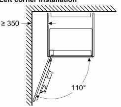
If using the  $92^{\circ}$  hinge limiter, the min. distance to the wall is only 100 mm
