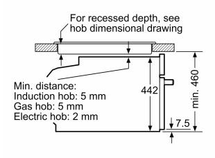
measurements in mm
