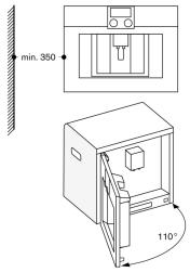
If using the 92  $^{\circ}$  door hinge restrictor (spare part no. 00636455), the minimum distance from the wall is only 100 mm.
