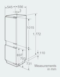
measurements in mm Recommended gap dimensions for flat hinges
