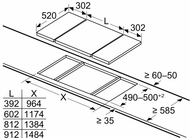
When installing two Domino units right next to a hob, two assembly kits (HZ394301) are required
