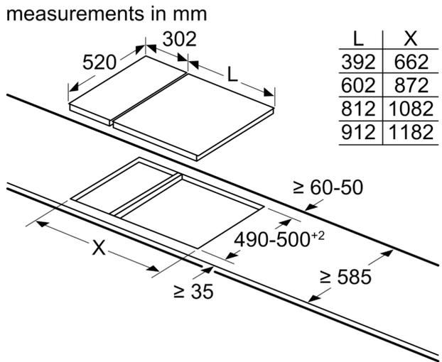
When installing a Domino unit right next to a hob, an assembly kit (HZ394301) is required.
