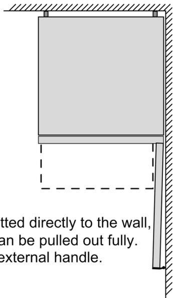
If the appliance is fitted directly to the wall,
