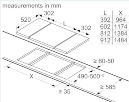
When installing two Domino units right next to a hob, two assembly kits (HZ394301) are required.
