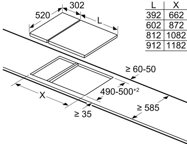
When installing a Domino unit right next to a hob, an assembly kit (HZ394301) is required.
