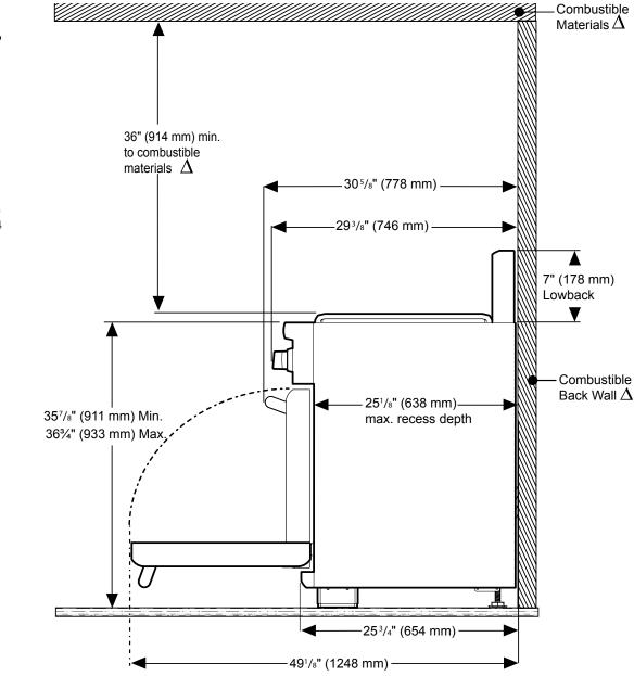
$\Delta$  As defined in the "National Fuel Gas Code" (ANSI Z223.1, Current Edition). Clearances from non-combustible materials are not part of the ANSI Z21.1 scope and are not certified by CSA. Clearances of less than 6" (152 mm) must be approved by the local codes and/or by the local authority having jurisdiction. Thermador
