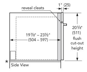
**NOTE:** \* Flush installation requires a 5/16" (8 mm) high x  $28\frac{1}{2}$ " (724 mm) wide x  $22\frac{1}{2}$ " (571 mm) deep baseplate underneath the unit body.
