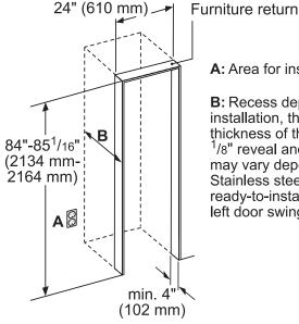
A: Area for installation of power connection.
