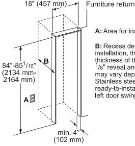
A: Area for installation of power connection.
