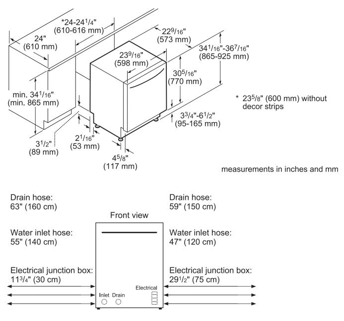
All connections are at the rear of the appliance. Extension for drain hose available as accessory. Power cord for connection to electrical outlet (3-prong plug) available as accessory.
