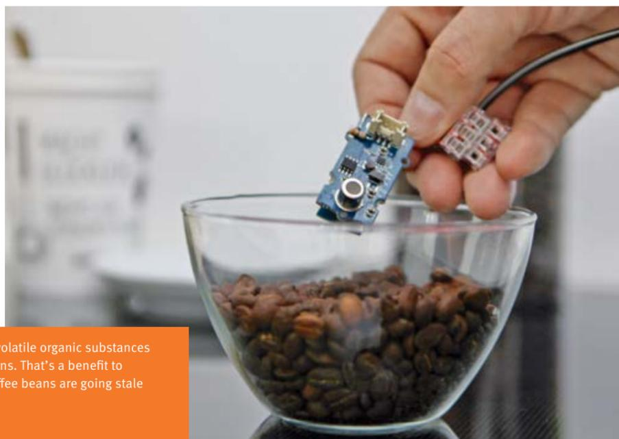
The Smart Smell "sniffer" detects volatile organic substances from food even at low concentrations. That's a benefit to consumers – for instance when coffee beans are going stale and should be used up soon.
