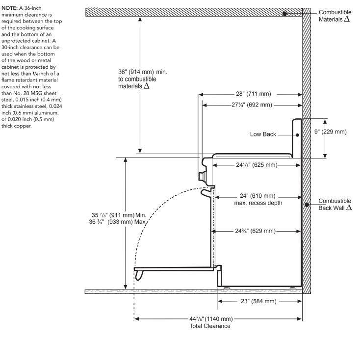
▲ As defined in the "National Fuel Gas Code" (ANSI Z223.1, Current Edition). Clearances from non-combustible materials are not part of the ANSI Z21.1 scope and are not certified by CSA. Clearances of less than 12" (305 mm) must be approved by the local codes and/or by the local authority having jurisdiction.
