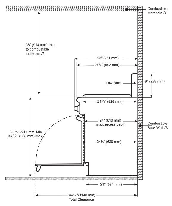
⚠ As defined in the "National Fuel Gas Code" (ANSI Z223.1, Current Edition). Clearances from non-combustible materials are not part of the ANSI Z21.1 scope and are not certified by CSA. Clearances of less than 12" (305 mm) must be approved by the local codes and/or by the local authority having jurisdiction.
