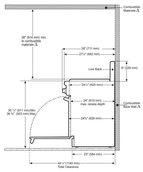
$\Delta$  As defined in the "National Fuel Gas Code" (ANSI Z223.1, Current Edition). Clearances from non-combustible materials are not part of the ANSI Z21.1 scope and are not certified by CSA. Clearances of less than 12" (305 mm) must be approved by the local codes and/or by the local authority having jurisdiction.
