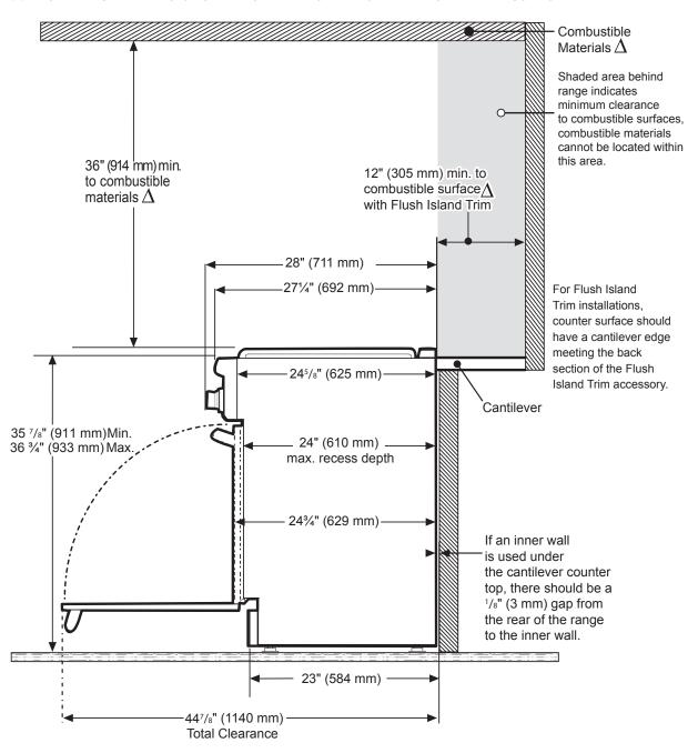
$\Delta$  As defined in the "National Fuel Gas Code" (ANSI Z223.1, Current Edition). Clearances from non-combustible materials are not part of the ANSI Z21.1 scope and are not certified by CSA. Clearances of less than 12" (305 mm) must be approved by the local codes and/or by the local authority having jurisdiction.
