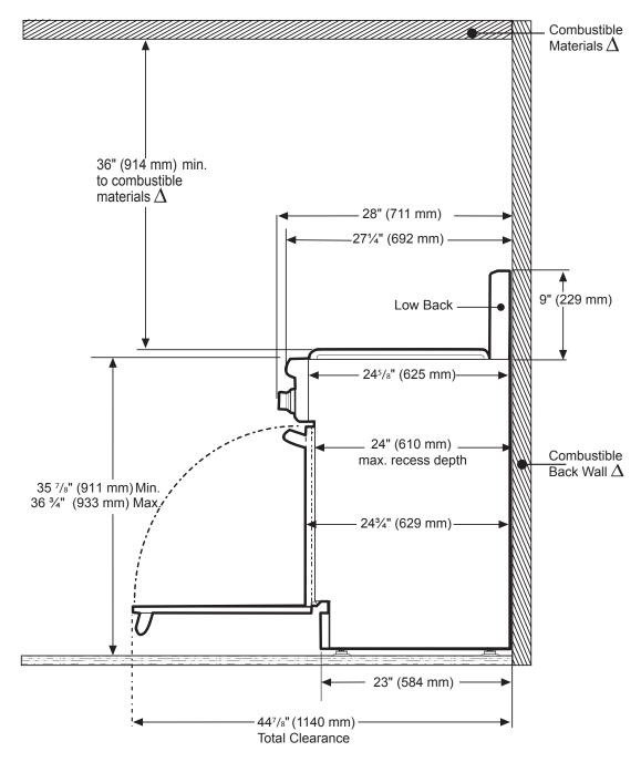
⚠ As defined in the "National Fuel Gas Code" (ANSI Z223.1, Current Edition). Clearances from non-combustible materials are not part of the ANSI Z21.1 scope and are not certified by CSA. Clearances of less than 12" (305 mm) must be approved by the local codes and/or by the local authority having jurisdiction.
