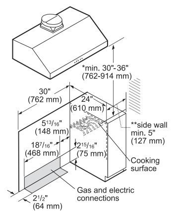
\* 30" (762 mm) minimum clearance above cooking surface to non-combustible surface. Minimum clearance above cooking surface to combustible surface is 36" (914 mm).
