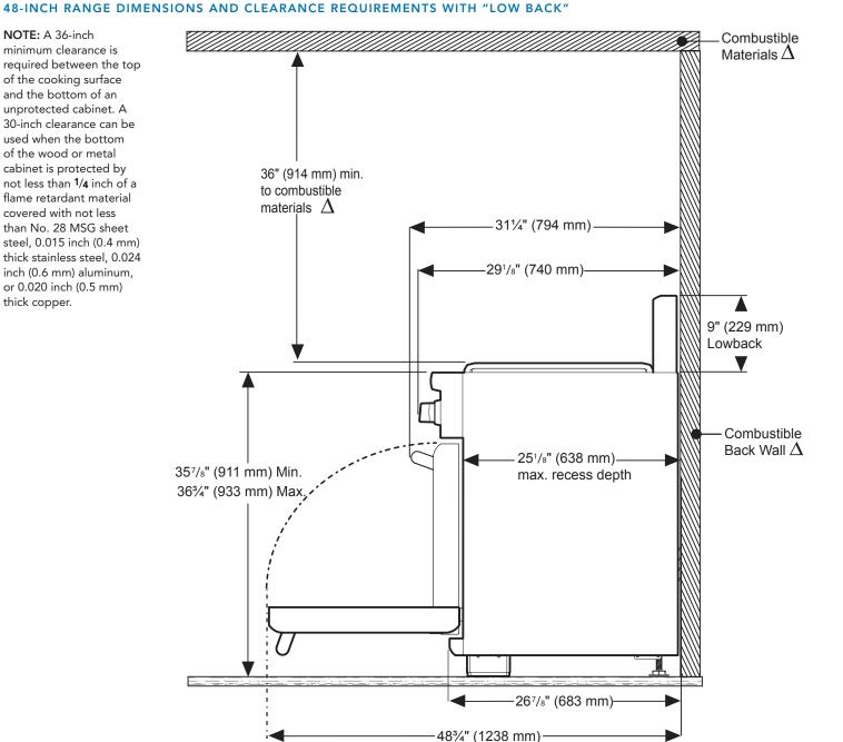
$\Delta$  As defined in the "National Fuel Gas Code" (ANSI Z223.1, Current Edition). Clearances from non-combustible materials are not part of the ANSI Z21.1 scope and are not certified by CSA. Clearances of less than 12" (305 mm) must be approved by the local codes and/or by the local authority having jurisdiction.
