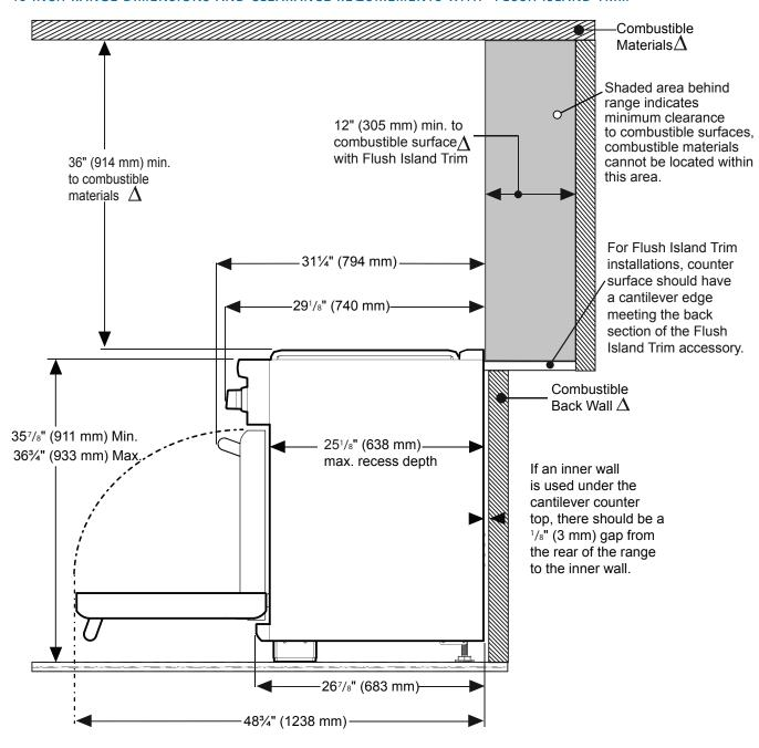
⚠ As defined in the "National Fuel Gas Code" (ANSI Z223.1, Current Edition). Clearances from non-combustible materials are not part of the ANSI Z21.1 scope and are not certified by CSA. Clearances of less than 12" (305 mm) must be approved by the local codes and/or by the local authority having jurisdiction.
