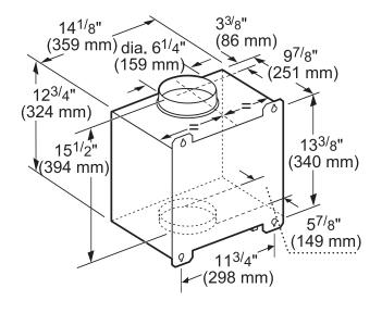
measurements in inches and mm
