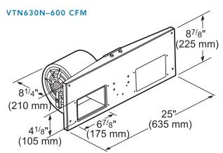
measurements in inches and mm
