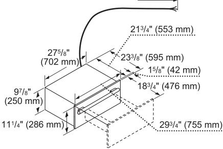
Note: 1 <sup>5</sup>/<sub>8</sub>" is the depth of the standard front panel (includes gasket). Dimension is not valid for custom panel product.
