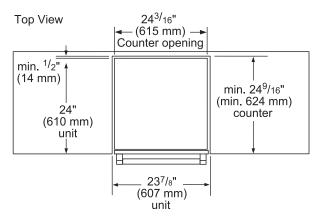
Thermador double drawer under counter top dimension. (Unit door flushed with the cutout)
