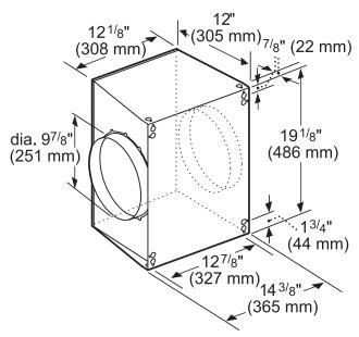
measurements in inches and mm
