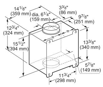
measurements in inches and mm
