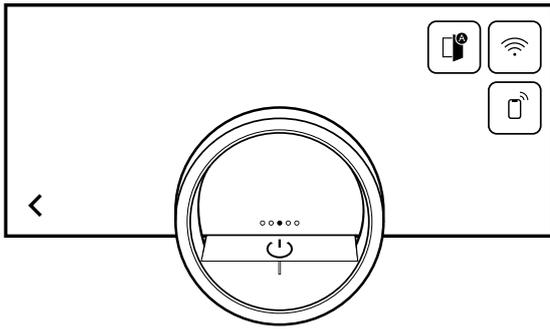
On the left-hand side, the display shows the symbols and texts with information on the current status of the appliance. On the right-hand side, the display shows the touch fields of the control centre.
