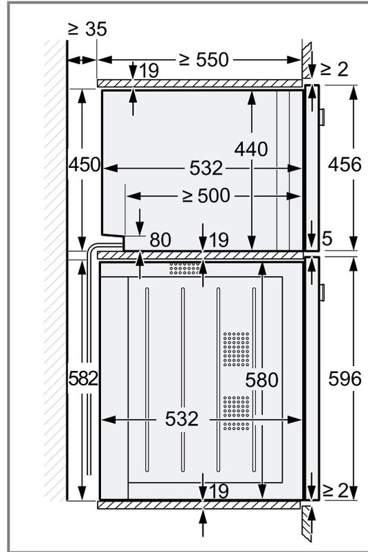
6. If there is no intermediate floor above the appliance, secure the appliance against tipping in the unit. Secure 2 commercially available brackets on both sides in the unit at a depth of 450 mm, 5 mm above the height of the appliance.
