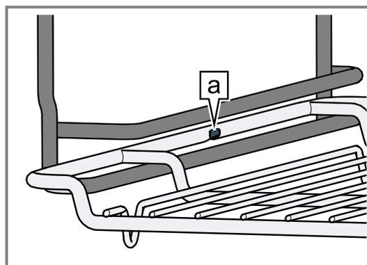
2. Ensure that the safety bracket on the wire rack
