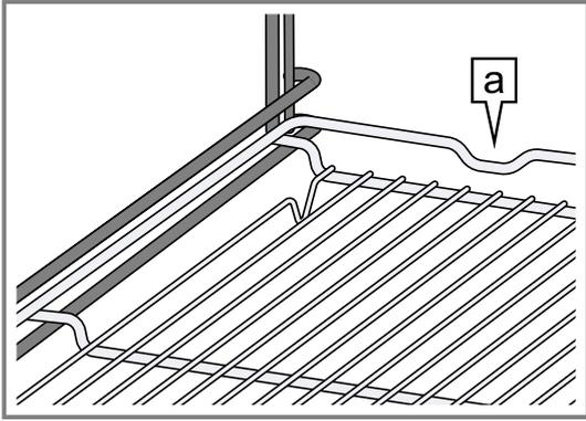
**Note:** To remove it completely, lift the wire rack slightly and pull it out with both hands. Remove any accessories that you do not require from the cooking compartment.
