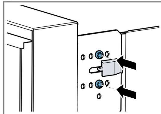
The further right you screw the screws into the appliance, the smaller the door opening angle. When the screws are positioned to the right, the opening angle of the appliance door is approx. 97°.
