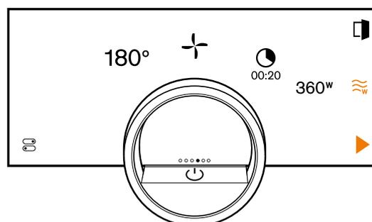
3. Add a microwave power level using ≈. You can also add the microwave operation while a heating process is active.
