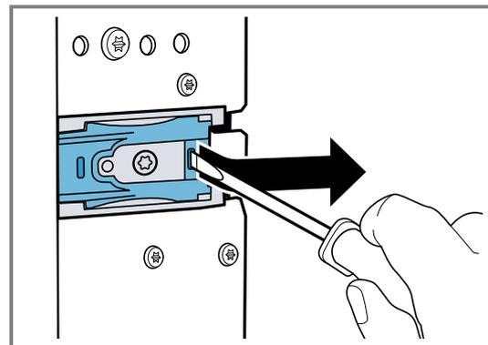
9. If the thickness of the side sections of the unit is 19 mm, remove the white plastic elements ①, turn them 180° ② and refit them ③.
