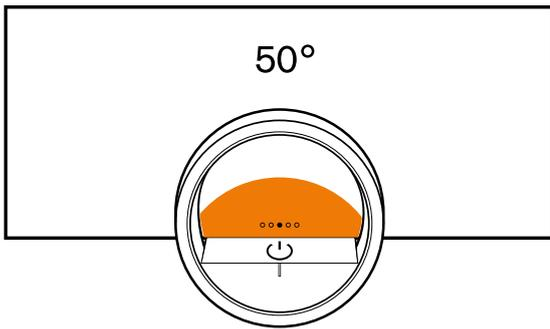
The section of the circle in orange becomes larger, the longer the timer runs or the closer the core temperature of the food approaches the set core temperature. If no cooking time and no core temperature are set, the section of the circle pulsates in orange.
