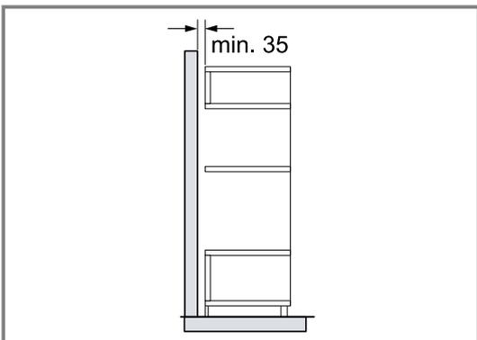
5. When installing 2 appliances on top of each other, observe the clearances.
