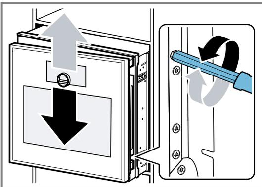
5. Tighten the two screws on the side of the appliance.
