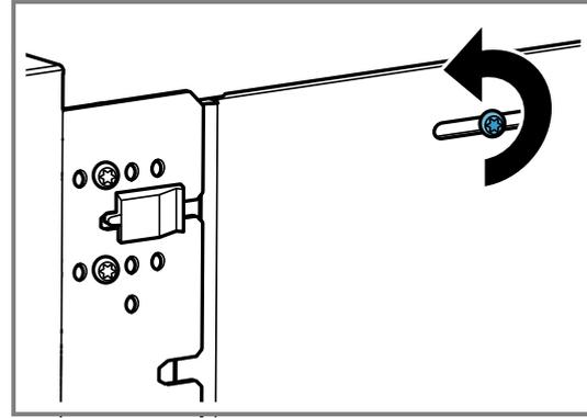
3. Remove the two screws in front of the black plastic element.
