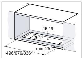
2. Make the cut-out for the exhaust air pipe either above the fitted unit or behind the fitted unit above the appliance.
