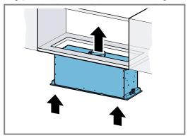
2. Tighten the two fastening screws alternating between the left and right. Use a suitable tool to avoid damaging the surface.
