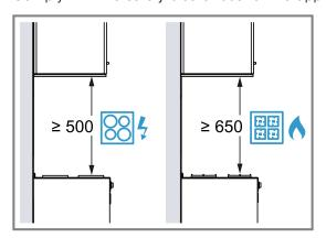
For Australia and New Zealand the minimum safety clearance above electrical cooktops must be 600 mm.
