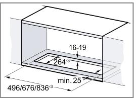
2. Make the cut-out for the exhaust air pipe either above the fitted unit or behind the fitted unit above the appliance.
