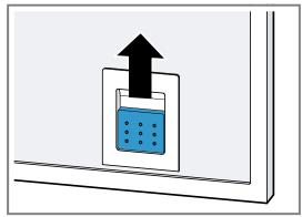
Remove the grease filters from the holders. To prevent grease from dripping, hold the grease filter horizontally.
