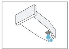
Check the condensation container filter regularly and clean the filter if it is dirty. → Page 44 Make sure that you insert the condensation container before operat-
