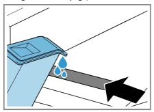
Observe the mark for filling the water tank next to the front opening. If  $\lozenge$  does not go out on the display, align the appliance correctly.  $\rightarrow$  "Aligning the appliance", Page 16
