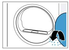
3. Remove the two-part fluff filter.
