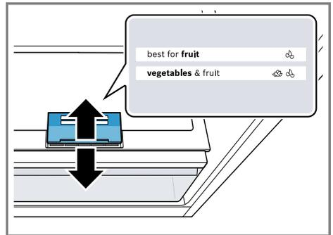
The air humidity in the fruit and vegetable container can be set according to the type and amount of food to be stored by moving the humidity controller:
