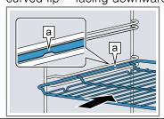
Tray E.g. universal pan or baking tray Slide the tray in with the sloping edge towards the appliance door.
