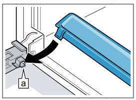
3. Slide the intermediate pane into the left- and right-hand retainers a.
