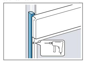
4. Secure the appliance using a suitable screw.
