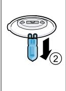
**4.** Insert the new halogen bulb and press it firmly into the socket.
