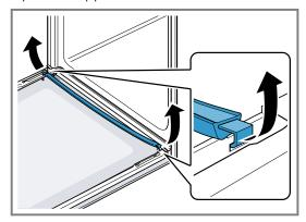
**8.** Lift out the intermediate pane and set it down carefully on a flat surface.
