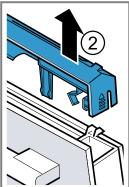
6. Lift out the inner pane and set it down carefully on a flat surface.
