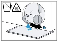
8. Firmly press on the sealing cap.
