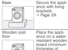
resistant wooden board (minimum thickness of 30 mm) which is screwed tightly to the floor.
