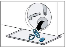
**3.** Ensure that both impellers can turn.
