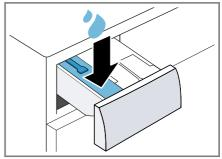
6. Add washing powder containing oxygen bleach to the manual dosing compartment.
