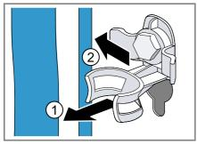
2 Unscrew ① and remove ② all of the screws for the 4 transit bolts using a WAF 13 wrench.
