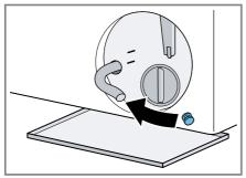
**9.** Insert the drain hose into the holder.
