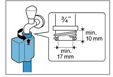
2. Open the water tap carefully and check that the connection points are tight.
