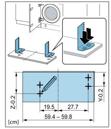
4. Note: When inserting the base panel, ensure that, if the base panel is protruding or the cabinet panel is flush-mounted, the time-Light is not visible.
