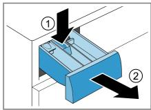
3. Pull out the insert upwards.
