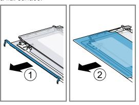
**9.** Loosen the screw on the left- and right-hand spacers ⓐ ① and remove both spacers ②.
