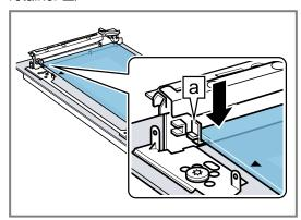
4. Slide in a second intermediate pane. When doing so, ensure that the number on the intermediate pane is at the bottom right 1.
