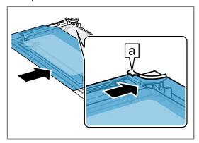
**10.**Push the inner pane upwards until it is in the left- and right-hand retainers a.
