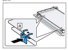
8. Secure the left- and right-hand spacers with one screw each.
