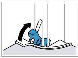
▼ The locking levers are closed. The appliance door is secured and cannot be detached.
