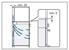
Only fit the appliance up to a height which allows accessories to be easily removed.
