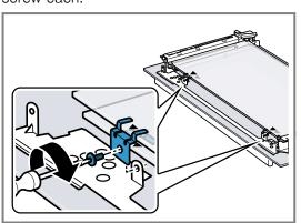
**9.** Slide the inner pane in. In doing so, ensure that the inner pane is in the retainer **a**.
