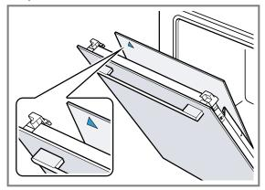
**1.** Slide the first intermediate panel into the lowest retainer ① and fit it at the top.
