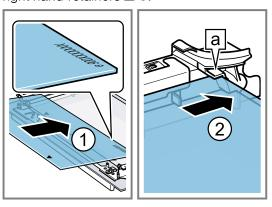
6. Push the intermediate pane upwards until it is in the retainer a.
