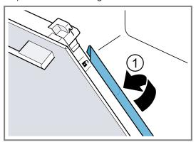
**4.** Slide the inner panel into the retainer at the bottom ① and fit it at the top.
