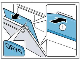
The lettering "Pyro" must be legible at the top, as shown in the picture.
