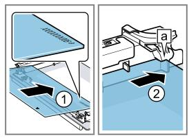
3. Push the intermediate pane upwards until it is in the retainer a.
