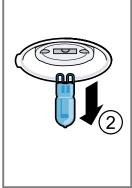
**4.** Insert the new halogen bulb and press it firmly into the socket.
