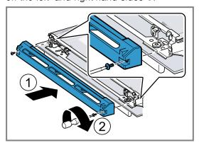
**13.Note:** Ensure that the appliance door slides onto the hinges without any resistance. If you feel any resistance, check whether you are sliding it in at the correct opening.
