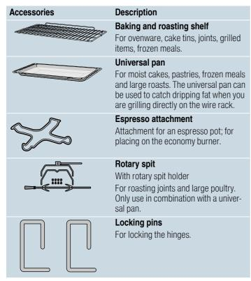
The baking tray and the baking and roasting shelf can be moved into five different heights within the cooking compartment. Always insert them as far as they will go so that the accessories do not touch the door panel. Ensure that you always insert the accessories into the cooking compartment the right way round.
