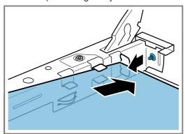
**2.** Hold the top pane in both brackets and insert it at an angle towards the back.
