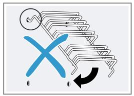
3. Both hooks must be inserted fully into the upper holes. Move the rail down slowly and carefully, and hook it into the lower holes.
