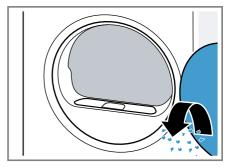
3. Remove the two-part fluff filter.
