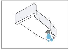
Check the condensation container filter → Page 38 regularly and clean the filter if it is dirty.
