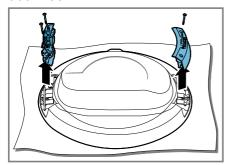
3. Screw the door hinge and the door hook onto the opposite sides.
