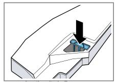
5. Insert the condensation container. → "Inserting the condensation container". Page 36
