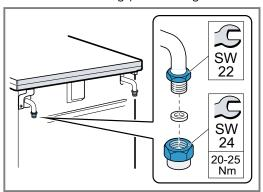
**3.** After changing the connection side, carry out a leak test. You can find additional information about this in the section entitled "Leak and function test" → Page 39.
