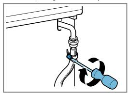
Open the gas connection shut-off. Carry out a leak test → Page 39.
