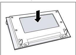
2. First tighten the two screws at the bottom again and then the two screws at the top.
