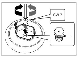
5. If your appliance features a wok burner with side access, remove the burner nozzle as shown below.
