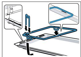
2. Slide the handle onto the rotary spit and screw it on
