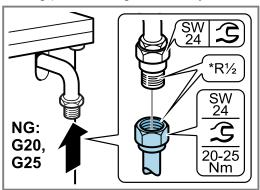
4. Open the gas connection shut-off. Carry out a leak test → Page 39.
