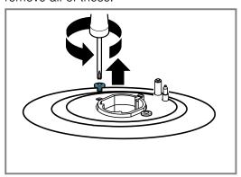
3. Undo the hob panel at the burner hub and lift it up.Pull the hob panel forwards.
