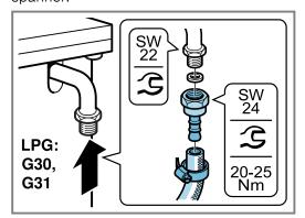
**3.** Fit the safety gas hose and use a pipe union or cable clamp to tighten it securely.
