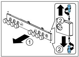
**6.** Remove the screws that become visible after you remove the knobs from the front panel.
