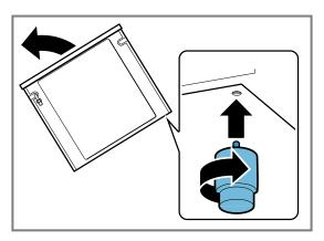
Note: If you then move the appliance, screw the adjustable feet in fully.
