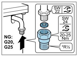
3. Secure the connecting piece using a 24 mm spanner. Use a 24 mm spanner to place the threaded fitting of the gas pipe or safety gas hose on the connecting piece and tighten it firmly.
