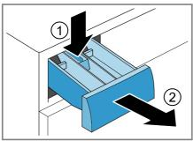
3. Pull out the insert upwards.
