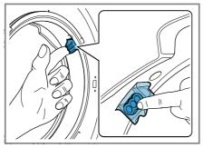
4. Clean the outside and the inside of the rubber gasket with a damp cloth and wipe dry.
