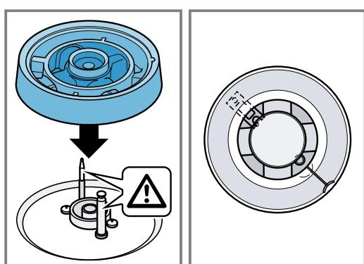
4. The locking catch on the burner ring must click into place in the corresponding recess on the burner head.
