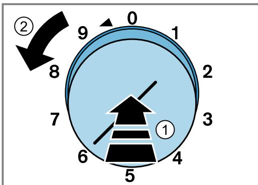
It can often be quicker to ignite the burner in the lowest setting because different gases have different ignition characteristics.
