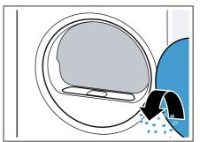
3. Remove the two-part fluff filter.
